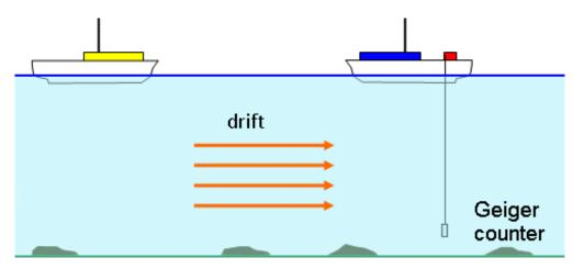
If a little radioactive material (usually iodine-131 with a half-life of 8.1 days) is put into a moving liquid the path of this liquid can be tracked. Used in testing blood flow, tracking underground streams and following the movement of silt in rivers.
