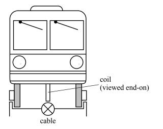
It is suggested that the force between a loop and a long current-carrying wire could be used in the design of a magnetically levitated train (Maglev). Many loops (a coil) are placed vertically in each carriage directly above a cable fixed to the track bed. If the dimensions are chosen so that a >> d and N is the number of loops in a coil then the force produced will be given by:
