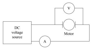
The motor was connected to a variable DC source as shown above. The voltage and current were measured when the coil was stationary and then five values of voltage and current were obtained with the motor turning. The rotation rate was measured using a strobe technique.
